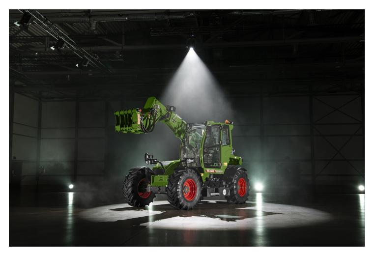
The new Fendt Cargo T740 telescopic loader has a lifting height of 7.70 m and a lifting capacity of 4 t in the class of 6 to 8 m working height. With this compact model, Fendt is pushing ahead with the volume segment, which occupies more than 80 percent of the European market for telescopic loaders.
