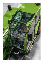
The oscillating control console is integrated on the right side of the driver's seat and allows maximum operating precision regardless of the operating environment. The colouring of the operating buttons corresponds to the Fendt logic, so users quickly find their way. In addition, the ergonomics and functions of the joystick were optimised.
