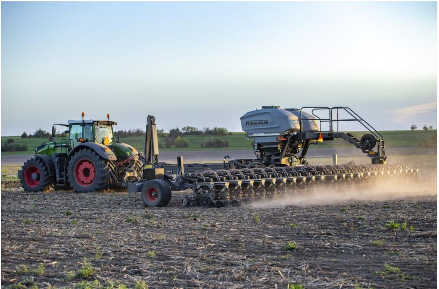
*The Fendt® Momentum™ planter from AGCO is the most agronomically advanced planter available worldwide and is designed to consistently place every seed at the optimum depth and spacing while minimizing compaction and eliminating pinch rows.*
